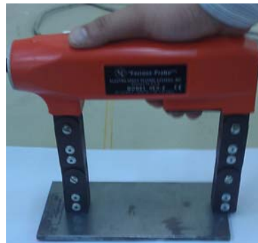
Fig. 9.16: Magnetizing the test piece.
