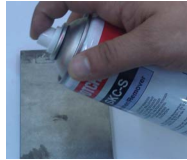
Fig. 9.15: Cleaning the test piece.
