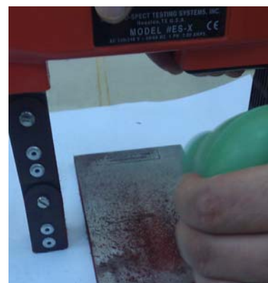
Fig. 9.18: Applying the dry magnetic particles.
