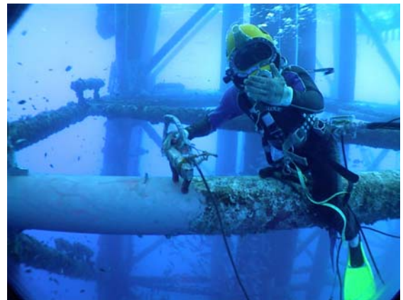
Fig 9.2: A Diver performing underwater magnetic particles test.
