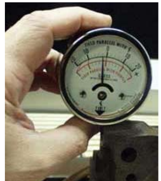
Fig. 9.14: Using a magnetic field indicator to measure the magnetic field.
