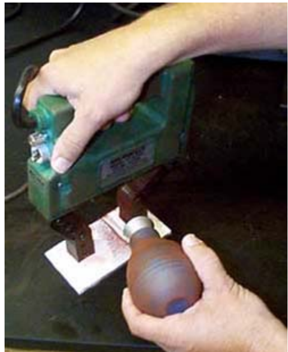
Fig. 9.11: Dry magnetic particles inspection.
