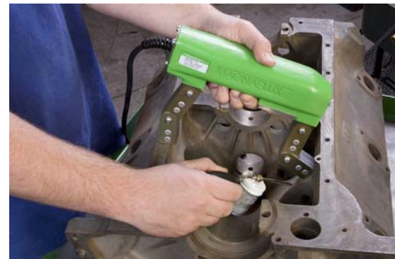
Fig. 9.13: Wet magnetic particles inspection.
