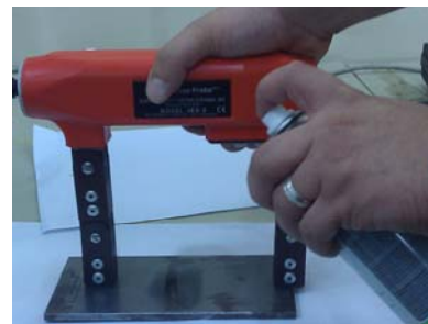
Fig. 9.17: Applying the wet magnetic particles.
