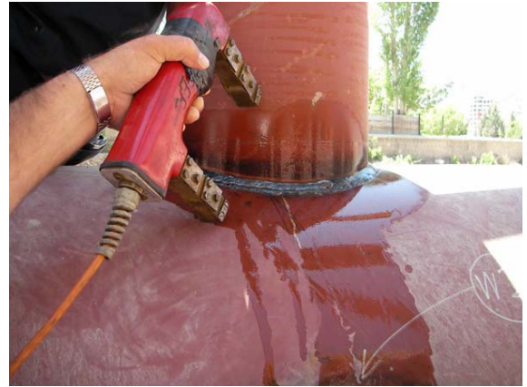
Fig. 9.1: Magnetic particles test of a weldment joining two pipes.
