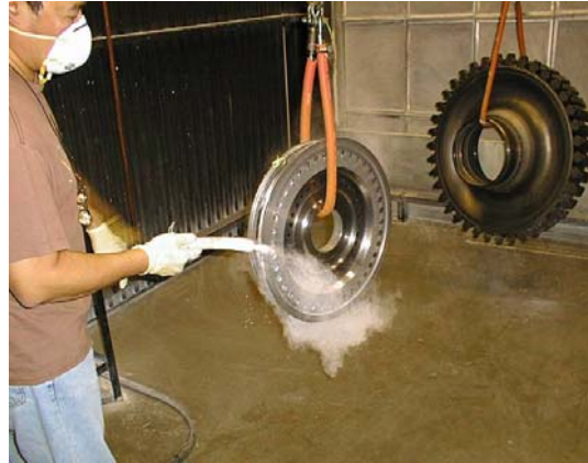
Fig. 8.7: Spraying the developer
