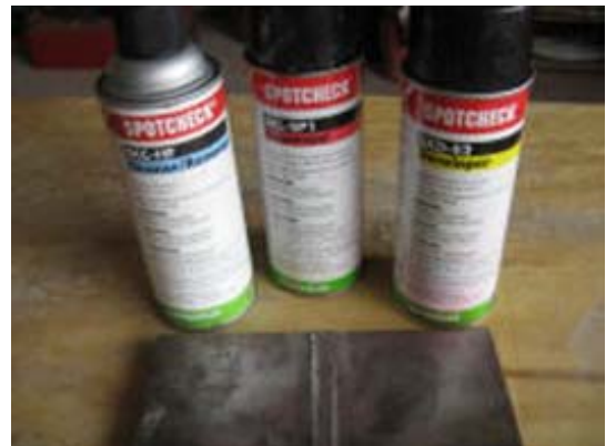
Fig. 8.10: The penetrant kit and the specimen.
