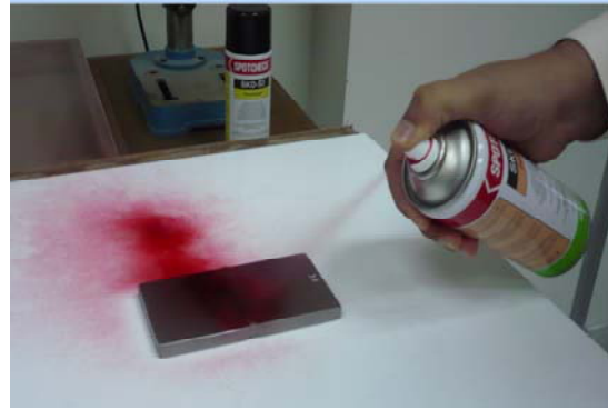
Fig. 8.12: Applying the penetrant.
