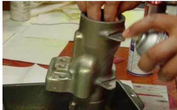
Fig. 8.4: Surface cleaning before the test.
