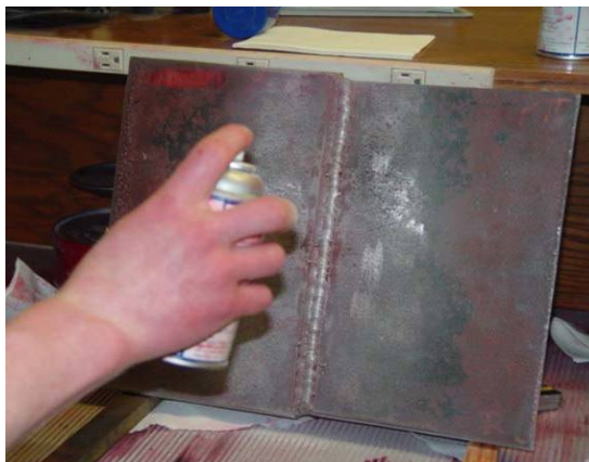
Fig. 8.14: Applying the developer.
