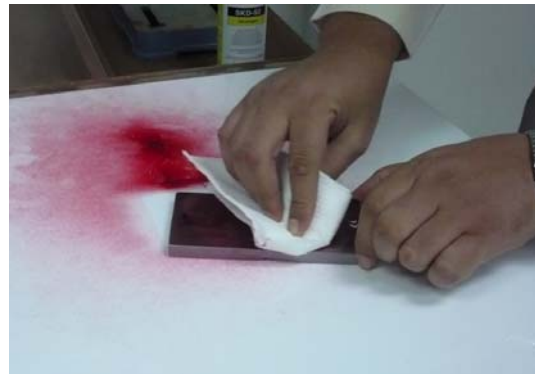
Fig. 8.13: Removing the excess penetrant.
