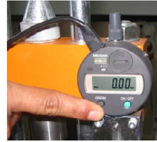
Fig. 5.9: Reset the DL-indicator.
