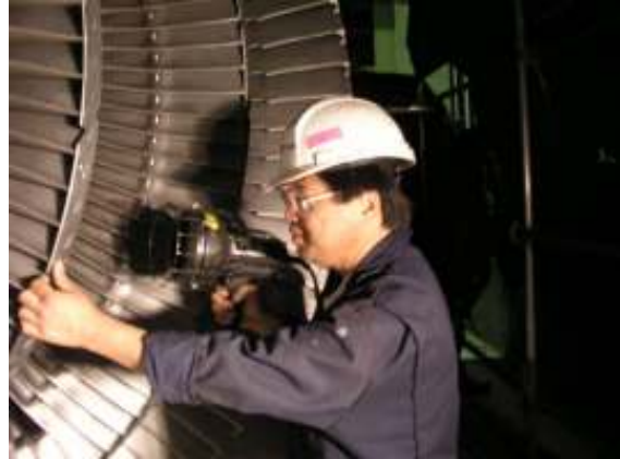
Fig. 3.5: A technician conducting a visual test.
