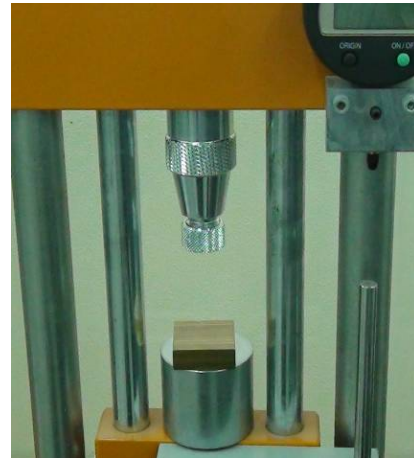
Fig.6.9: Place the test piece on the anvil.
