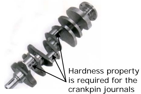
Fig.6.1: crank shafts need hardness property to resist wear
